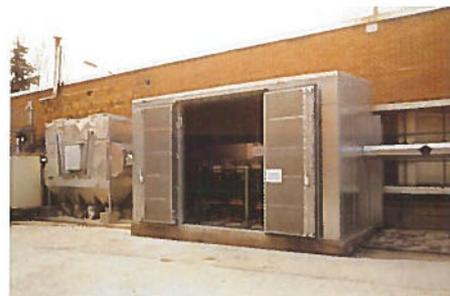
Pilot Plant Acoustic Preconditioning of Coal Combustion Emissions
